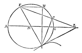
count of the conic Section is a right one <sup>2</sup>, so that FGL is one continued right Line, and IF is to IL as FG to GI; as likewise, M being the Center of the Circle, MI to IL, or FH to HI, as FG to twice GI, because MI is to IF as GI to twice GI. Hence by Permutation FH is to FG as HI to twice GI; that is, as the Sine of the Angle of Incidence to twice the Sine of the refracted Angle.
